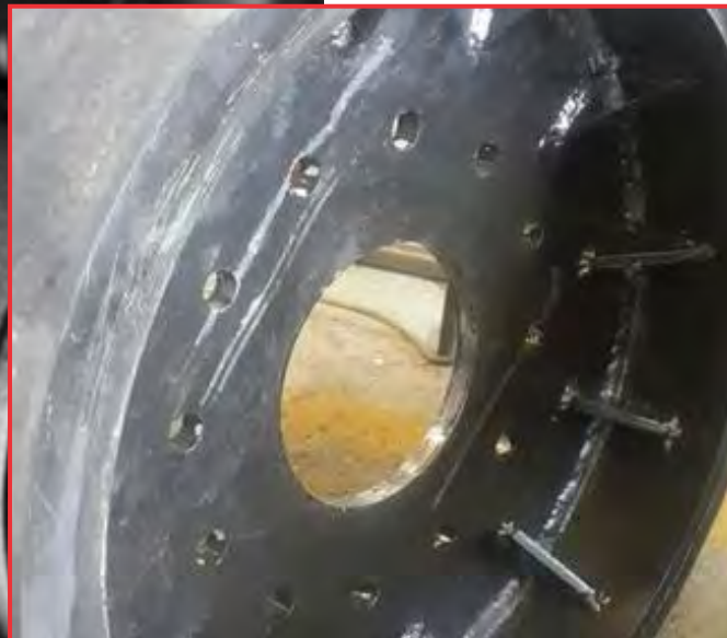
700MM DIAMETER WHEEL WITH BOUNDED 25MM RUBBER LAYER, 200 MM WIDE
